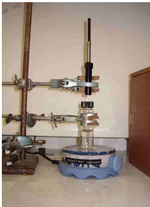
Figure 12. SPME method used to adsorb volatiles from the headspace. The solution was stirred to create a vortex during the 5-minute adsorption period
