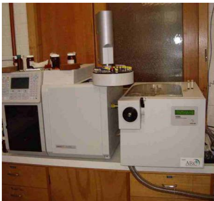
Figure 13. Varian 1200 Triple Quad GC/MS used to detect DMN
