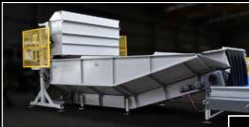
electric bin tipper & moving floor hopper
