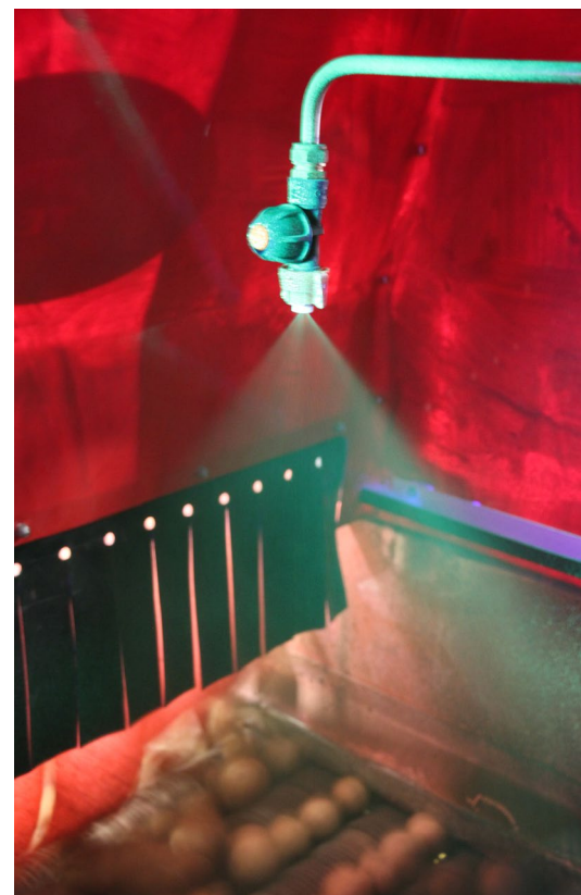
Using food-grade UV dye to assess the effectiveness of applicator coverage with a Syngenta VIBRANCE® Premium applicator.
