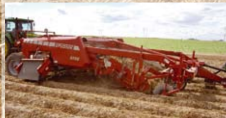
Spudnik MDL6140 4 row windrower with deviner web cushioned webs options available single row pick up and wheel drives.
