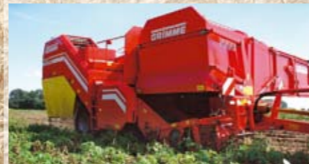
SE75-55 Featuring 5.8 tonne bunker, pre-cleaners, grader rollers, axle leveling and video monitoring.
