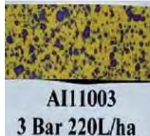
Figure 1: Water-sensitive paper showing spray coverage and pattern from different nozzles. Adjustment to water volumes and nozzle orientation can improve coverage and spray penetration, whilst reducing potential for spray drift.
