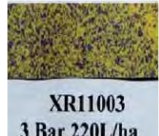
Figure 1: Water-sensitive paper showing spray coverage and pattern from different nozzles. Adjustment to water volumes and nozzle orientation can improve coverage and spray penetration, whilst reducing potential for spray drift.
