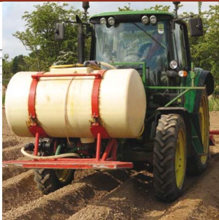
Front mounted liquid fertiliser tank for placement after planting. There is a small advantage to placement over broadcasting
