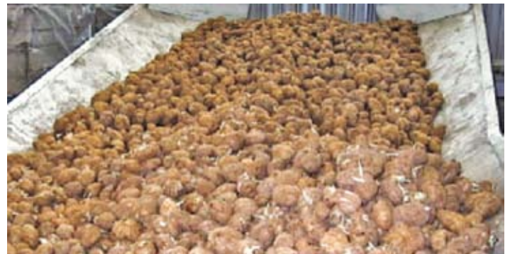
A well set up creep feed is an excellent way to handle seed potatoes, but steel surfaces should be rubberised to protect tubers from damage due to dropping and rolling.
