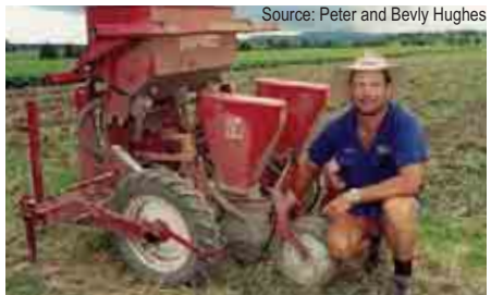
Below: Martin Wilson points out the Confidor application jet retro fitted to his bean planter.
