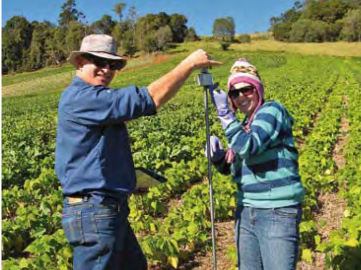
DPI&F horticulturist John Bagshaw and DPI&F microbiologist Lisa Gulino operate the hammer penetrometer during a cold winter's day in Gympie. The penetrometer measures the amount of force required to penetrate the soil, which is an indication of soil compaction.
