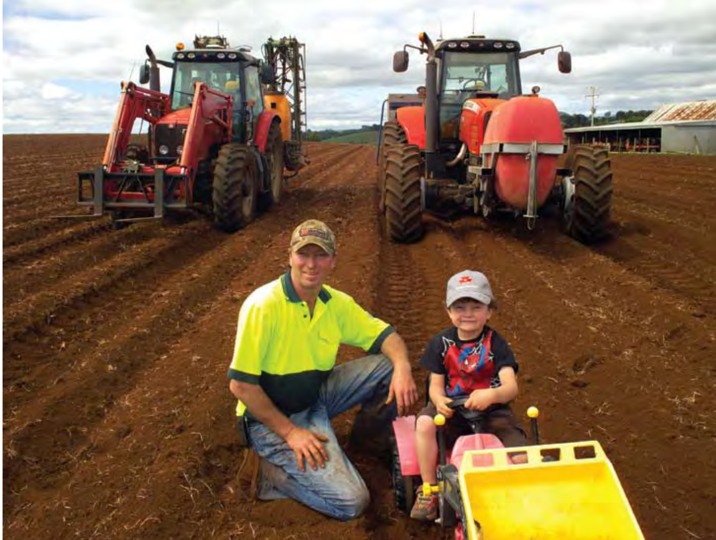
John McKenna, pictured with son Sean, has two tractors he uses on-farm—a 1.6 m track-width tractor [left] and 2.5 m model [right]. While the 2.5 m model is not integrated with the current CTF work, it does straddle three rows, which means that the middle row has no wheel tracks beside it.
