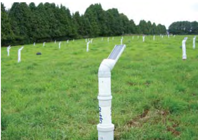
Wireless sensor network nodes [pictured above at a pasture in Elliot, Tasmania] will monitor soil moisture levels in real time to enable irrigation equipment to respond to soil-moisture variations across a vegetable crop. Image supplied by Tasmanian ICT Centre.
