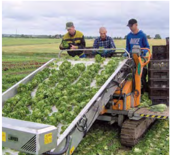
Ortomec's SVC Herbex is a tracked self-propelled harvester suitable for rapid harvesting in the field. It uses a single-blade cutting system, with oscillating movement. Image supplied by Tim Harslett.
