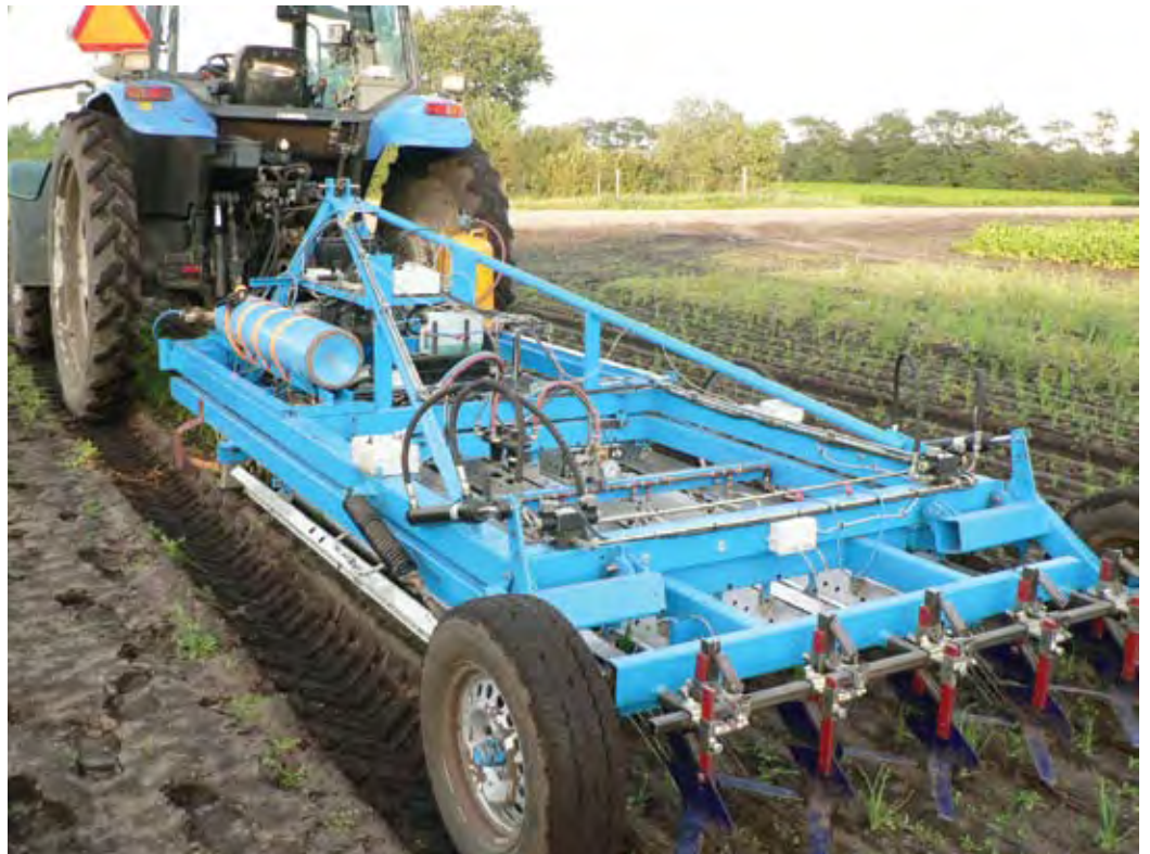
Vision Weeding's intra-row flame-weeder, available later this year, aims to provide efficient and economical weed control without herbicides. A computer, with an attached camera, detects individual plants within rows while the software calculates the plants' positions. The Plant Detection algorithms can distinguish between the crop and weeds, resulting in weeds being destroyed while crops are spared. Image supplied by Frank Poulson.
