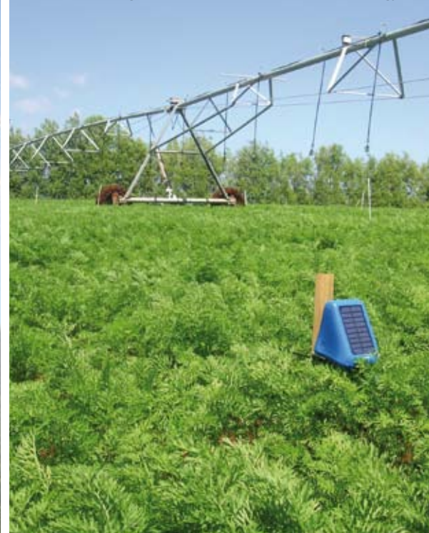
Linear move irrigator fitted with variable rate technology
