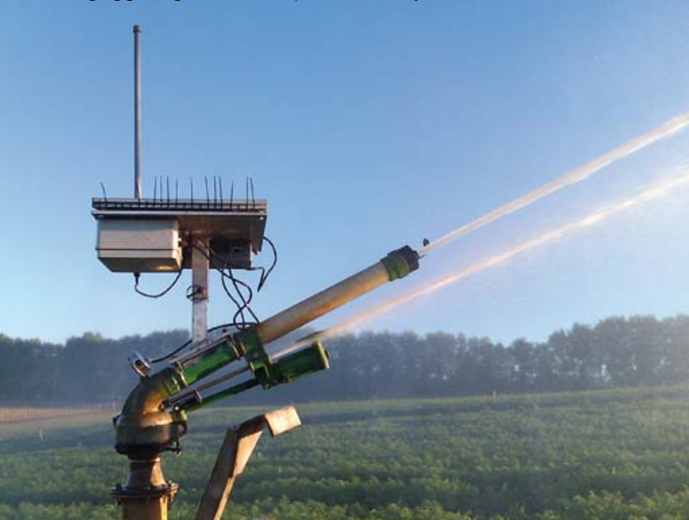
Travelling big gun irrigator fitted with a pressure control system
