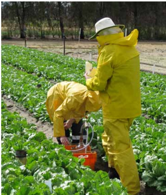
Pumping lysimeters in an iceberg lettuce trial, a weekly operation.
