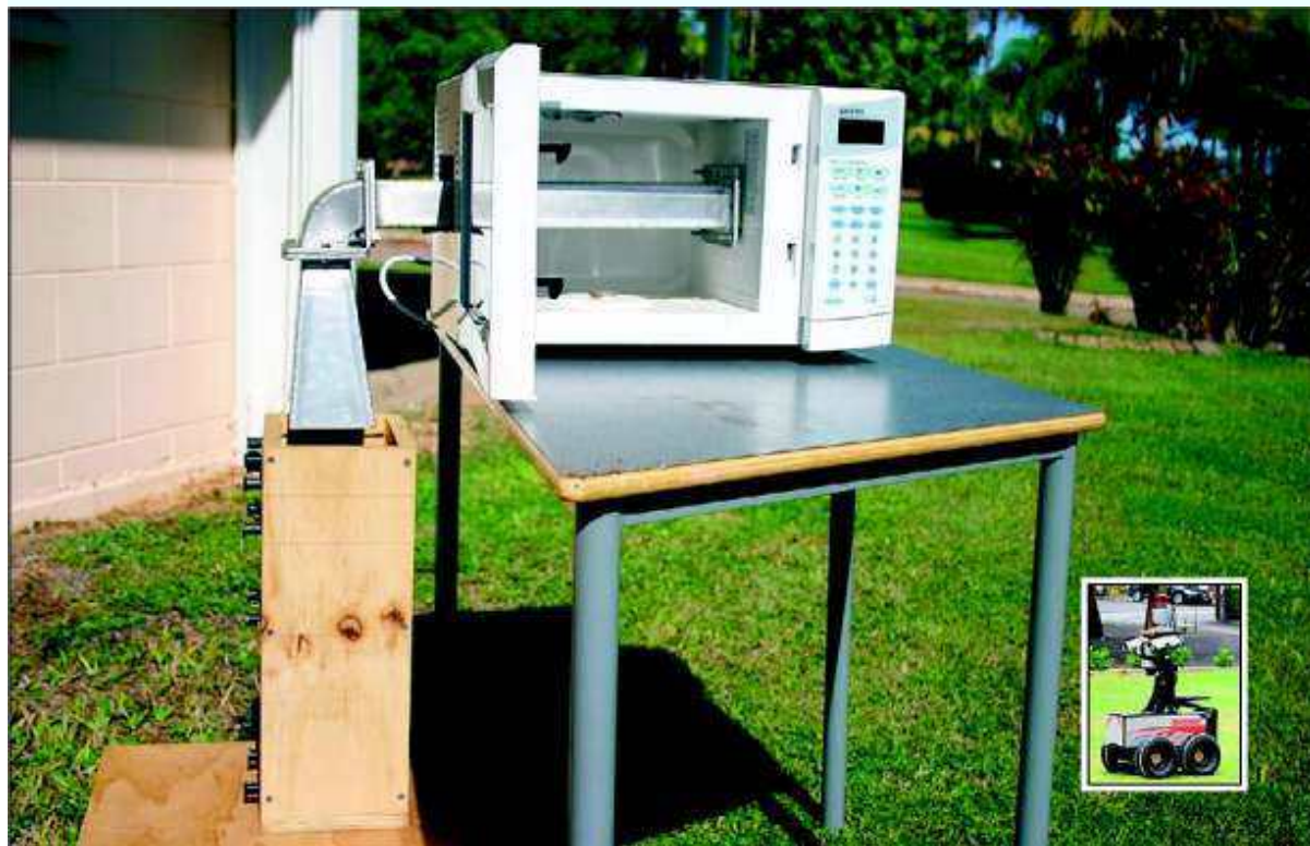
Microwave technology is being tested as a new form of selective weed control, main, and a shrimp device, inset
