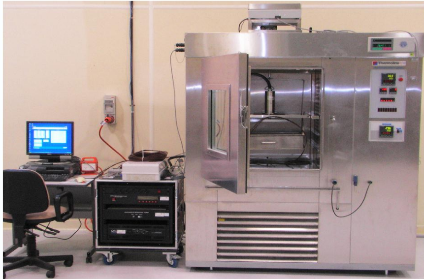
Photo of the ultrasonic-assisted test dryer
