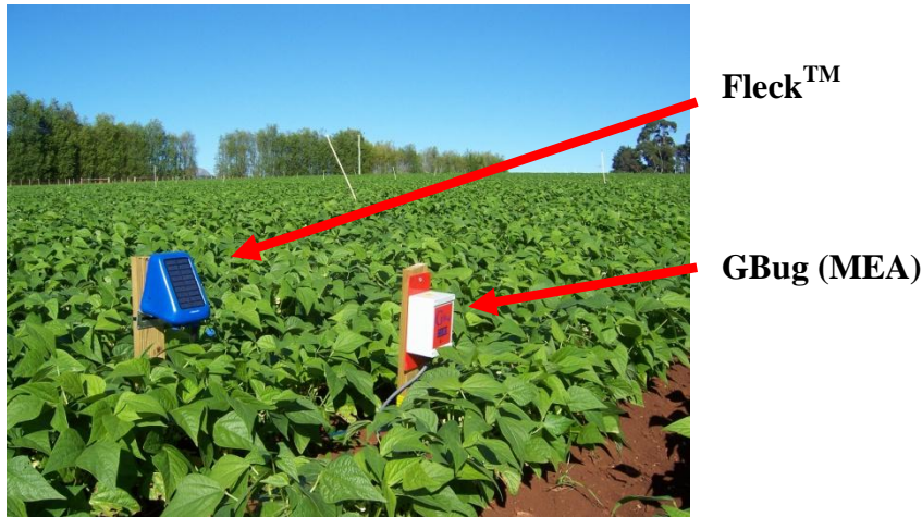
Figure 2.5. Photo showing Fleck™ (CSIRO ICT) and GBug (Measurement Engineering Australia) in green bean crop during 2010 season.
