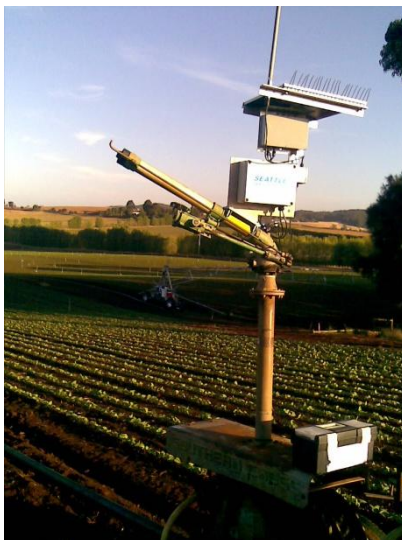
Figure 2.2. Pressure control system: a) prototype fitted to the soft hose irrigator (2010 season) and b) beta prototype fitted to a hard hose irrigator used in 2011 and 2012 season.
