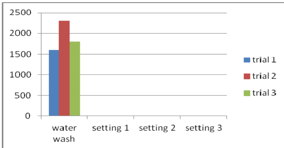
Figure 28; Graph showing the CFU per ml left in the wash in three separate trials using potable water to wash the leaf, potable water three settings of Unipolar disinfected water corresponding to 20ppm, 45ppm and 60ppm of disinfectant.
