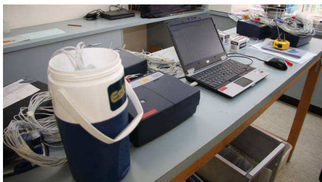
Figure 4.1 - Calibration of the temperature probes in a slurry of melting ice made from distilled water
