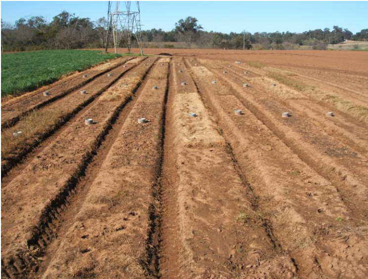
Image 5: View of the trial site before crops were transplanted. Note the size of plots and the placement of static manual gas chambers.
