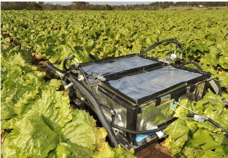
Image 1: Example of a gas-sampling chamber placed in a lettuce crop at Grech Farms. Note the doors are normally open, and close briefly to collect gas samples.
