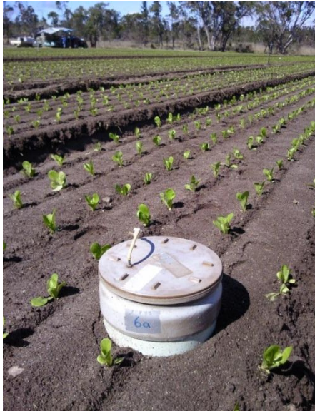
Figure 40. A measurement chamber deployed on-site in a crop of mini cos lettuce, first measurement campaign, September 2010, Granite Belt. The sampling tube and stopcock are clearly visible.
