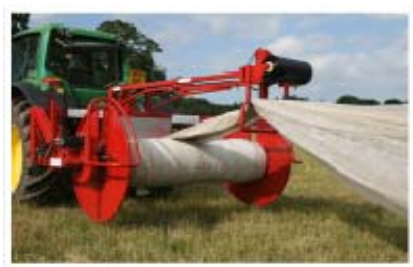
[Images 8, 9 & 10 – Tractor mounted commercial Crop Cover laying & retrieval device in UK]
