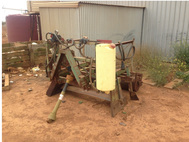
Figure 3-1: An applicator used to inject Metham Sodium into the soil at a farm at Werribee, Victoria
