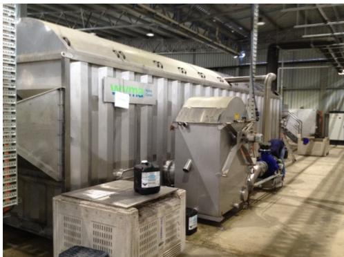
The flume channel shown below takes carrots from polishing to the hydro-cooler. VSDs are used on all electric motors, the polisher and the hydro-cooler to control flow rates while saving energy. The entire plant is remotely controlled allowing the hydro-cooler to do the bulk of its work during off-peak times.
