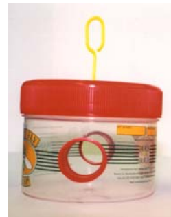
Figure 21. Modified Bugs for Bugs trap: - 2x 30mm diameter holes in entry ports
