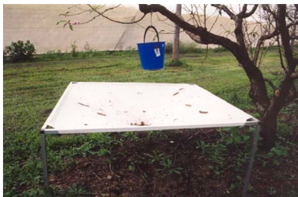
Figure 18. Collection system for assessing MAT carriers. Test devices attached to bucket handle at suspension point.
