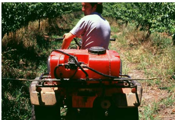
Figure 14. Quad bike with Silvan Rakpak fitted with Shurflo Pump.
