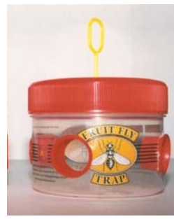
Figure 23. Modified Bugs for Bugs trap: - 4 x 30 mm diameter holes in entry ports
