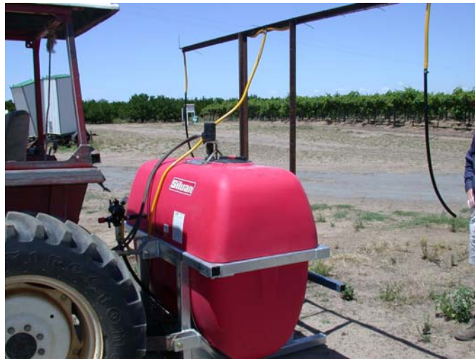
Figure 12. 1000L spray-vat, tractor drawn, for thickened fruit fly bait application. Note the in-tank stirrer for mixing the bait.
