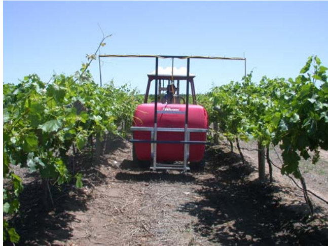
Figure 15. Applicator for thickened fruit fly bait being used in grapes at Emerald. Note the 1000L tank, in-tank stirrer, paired drip hoses for dripping/wiping the bait on the vines.
