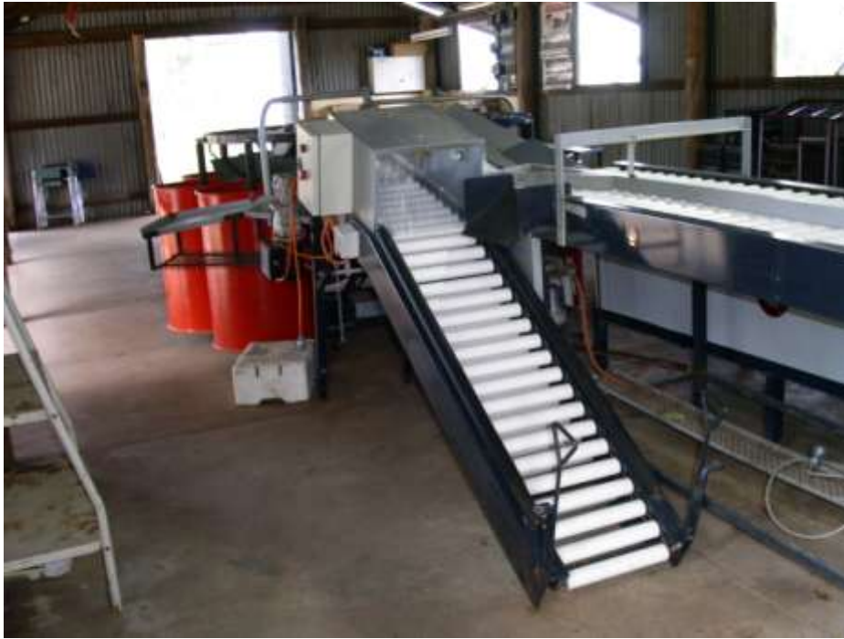
Figure 3. If required, fruit emerging from the dip can be treated with a flood spray (for fruit fly) which is contained in the box at the head of the rollers.
