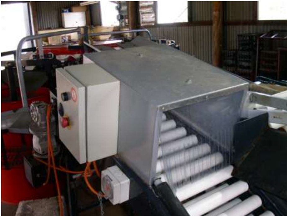
Figure 3. If required, fruit emerging from the dip can be treated with a flood spray (for fruit fly) which is contained in the box at the head of the rollers.
