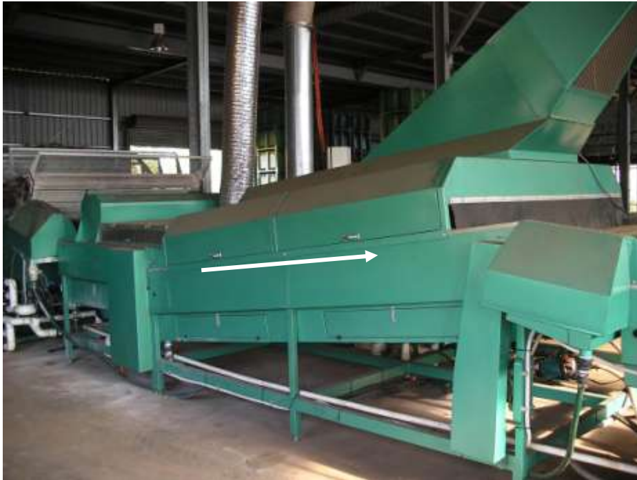
Figure 7. Following fungicidal treatment the fruit is then treated in a flood spray system. The treated fruit then moves in the direction of the arrow to air dry before grading and packing.
