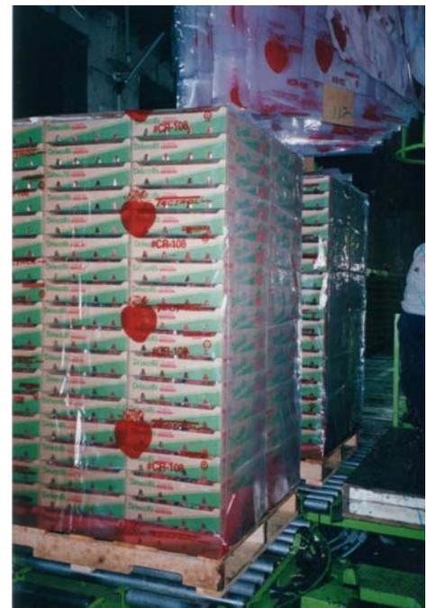
Photo 2. Bagging pallets for CO<sub>2</sub> injection
