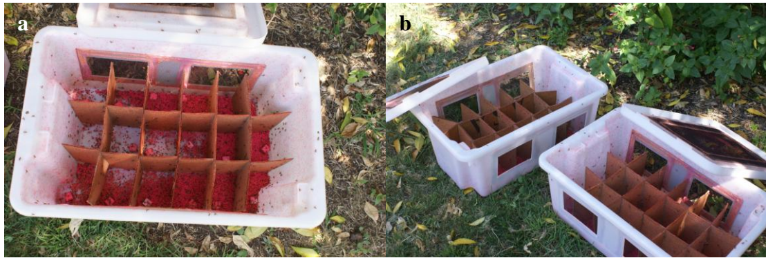
Figure 10. PARCs with cardboard inserts, showing sugar cubes in the base (a) and cardboard inserts (a & b).
