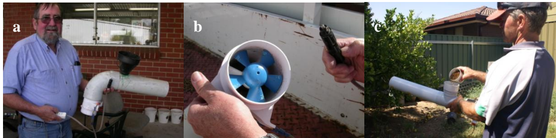
Figure 12. A prototype automated blower (a & c) that is run by a small fan and can be plugged into a car (b) or a battery pack (c) (battery not shown) to release chilled adult fruit flies.
