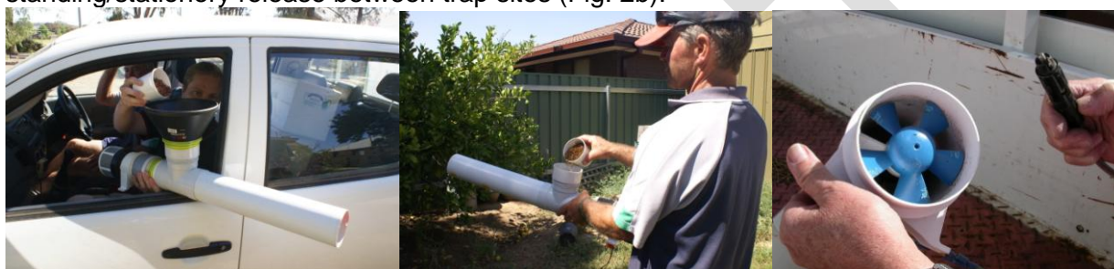
Figure 2. An automated blower (a & b) that is run by a small fan (c) and can be plugged into a car (c) or a battery pack (battery not shown) to release chilled adult fruit flies via roving (a) or stationery (b) release.
