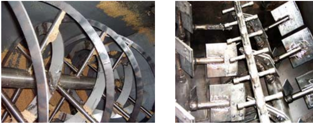
Figure 15: Horizontal ribbon and paddles mixers used to mix feed ingredients.
