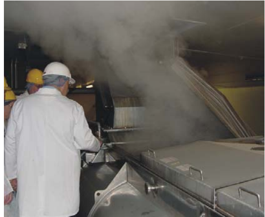
The high-pressure steam peelers.
