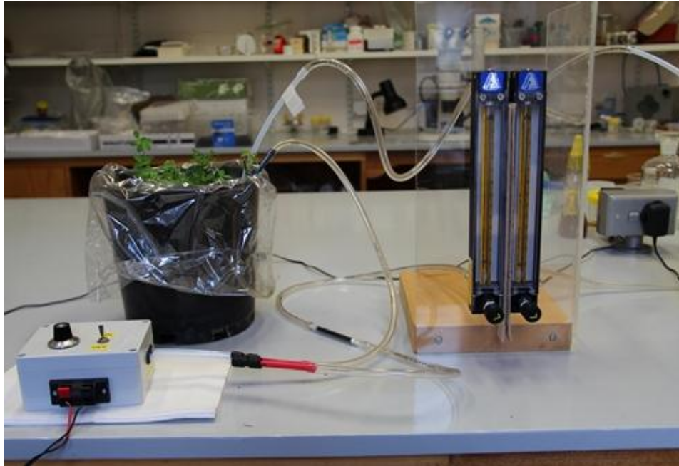
Fig. 7. Closed-loop air entrainment system used to collect plant root volatiles.
