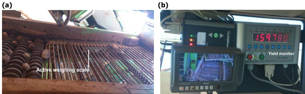
**Figure 2. Yield monitoring system components (a) active weighing scale (b) in-cabin monitor.**
