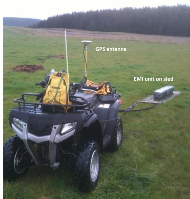
**Figure 1. Field survey vehicle and instruments to measure soil ECa (electro-magnetic induction (EMI) unit), and elevation (differential GPS).**
