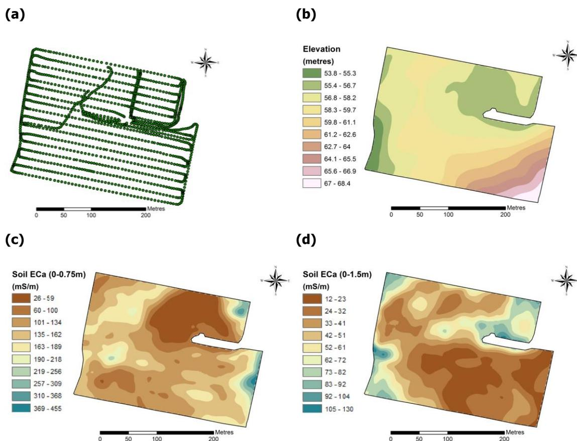
**Figure 3. An example of field survey data gathered using an ATV equipped with EM38DD and DGPS. (a) survey path, (b) mapped elevation, (c) soil ECa (0-0.75m), (d) soil ECa (0-1.5m).**
