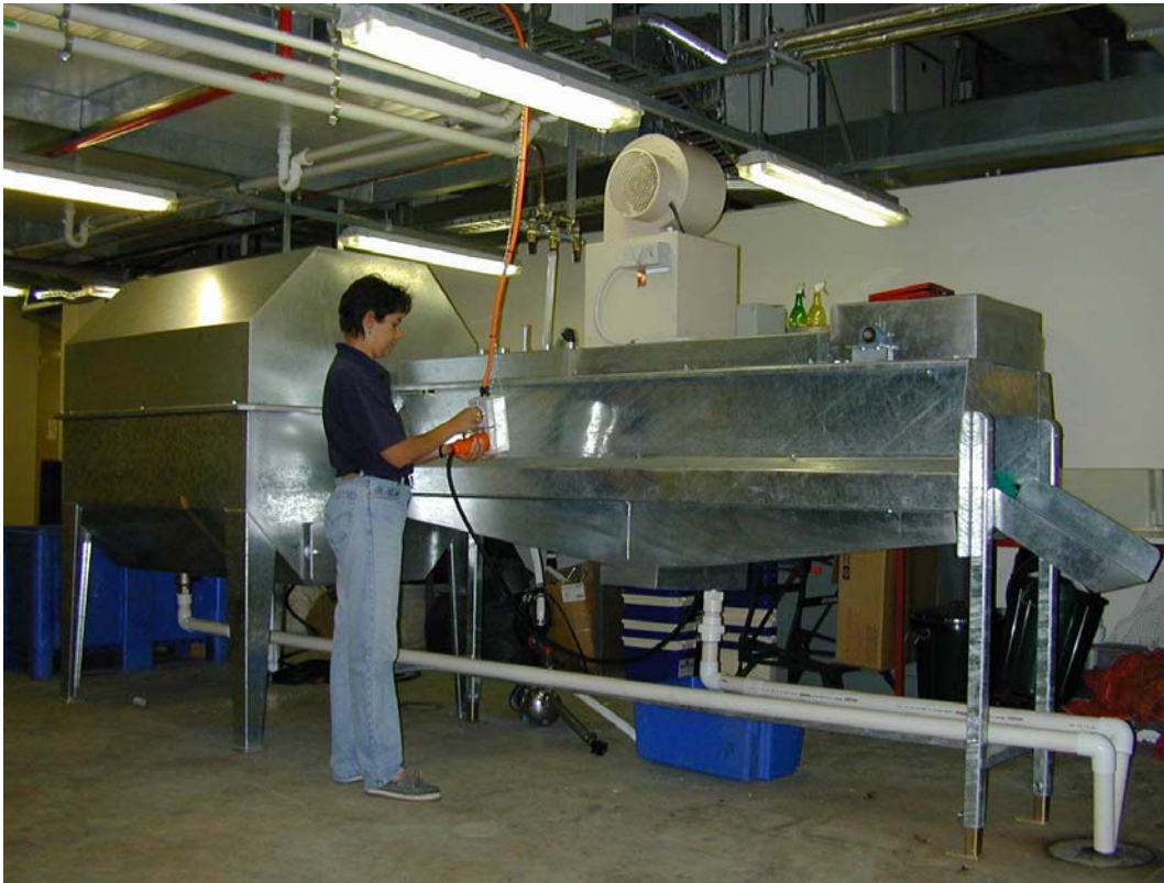
Figure 1 Mini Potato Washing Plant - Plant Research Centre
