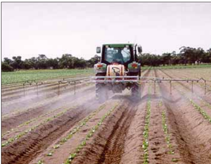
Droppers on a conventional boom help direct the spray into the canopy from multiple angles.
