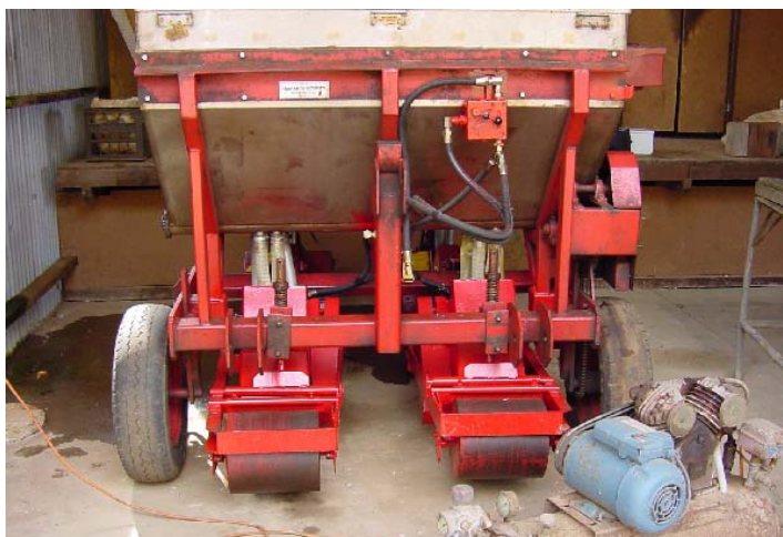
Figure 21: Grower built banding machine (attaches to planter), Manjimup, WA.
