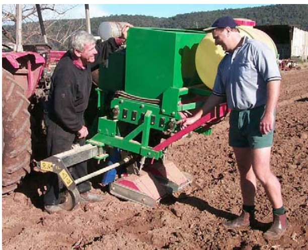
Figure 29: Precision incorporation machines designed to incorporate products into the transplant rows for improved clubroot control.
