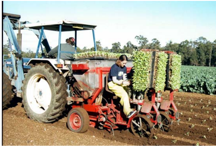
Figure 37: Grower designed and built modified planter in use – Manjimup WA.
