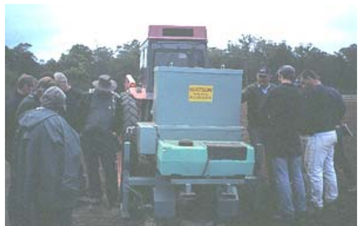
Figure 29: Precision incorporation machines designed to incorporate products into the transplant rows for improved clubroot control.
