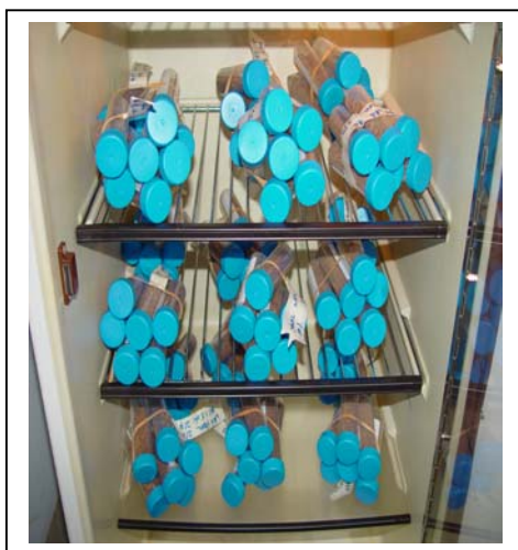
Plate 3: Inside incubator (37°C)- samples for pathogen re-growth trial.
