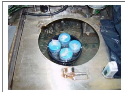
Plate 2: Inside chamber – plastic pot with sample tubes in water bath.
