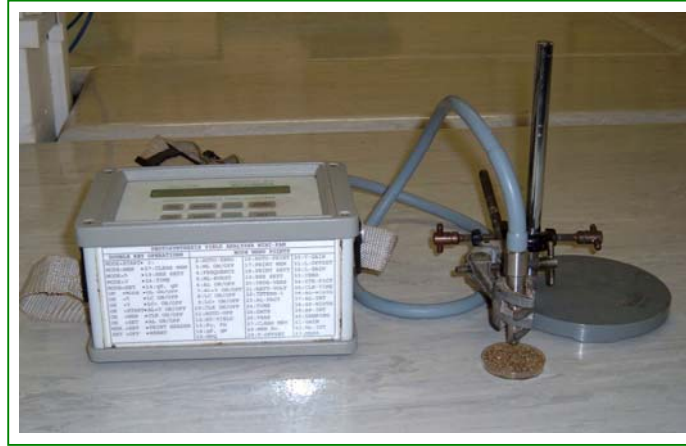
Plate 5.1 – PAM fluorometer set up for chlorophyll fluorescence measurements of carrot seed
