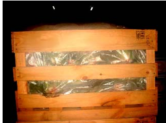
Figure 7.5.3. Sealed plastic top of half bin post transport, note upward bulging of plastic.
