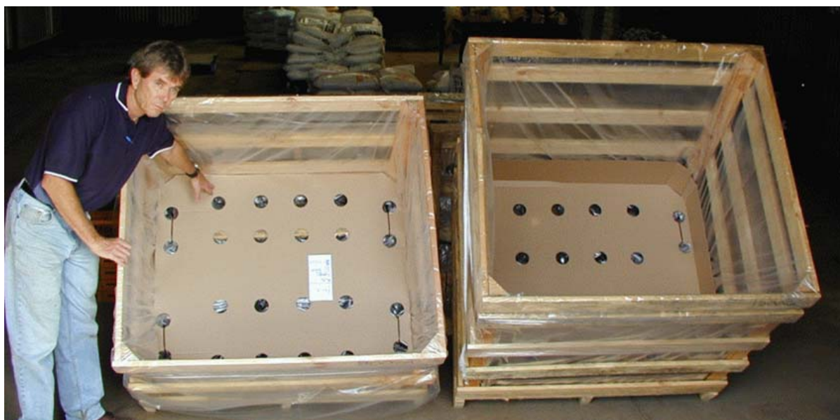
Figure 4.1. Bulk handling bin prototypes. Half bin on the left, Full bin on the right.
