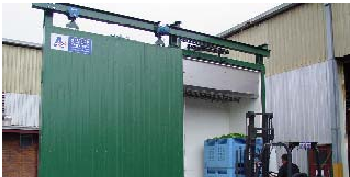
Figure 5.3.1. Vacuum cooler used to pre-cool sweetcorn in commercial cartons and bulk bin treatments.
