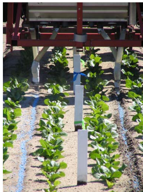
Figures 10.1a,b Banding Nitrophoska Blue Special ® by machine to main plot treatments.
