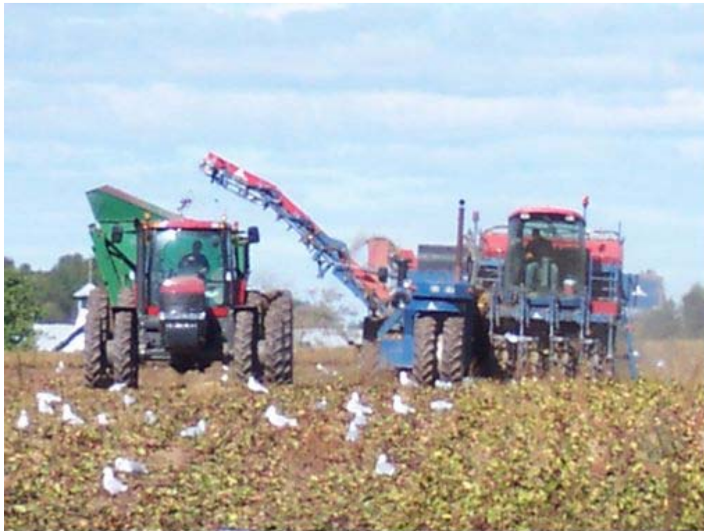
Myron Kudics farm USA - Four row new ASA Lift top lift harvester
