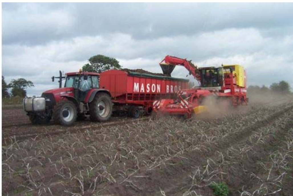
Stan White Farms UK - Shear lift harvester used for both Beetroot and Potatoes
