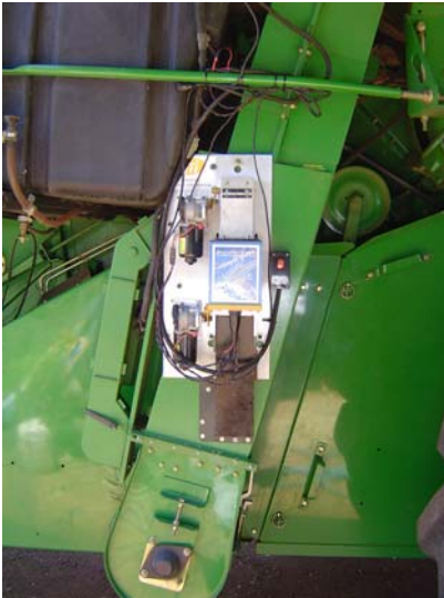
Protein Sensor mounted on clean grain elevator
