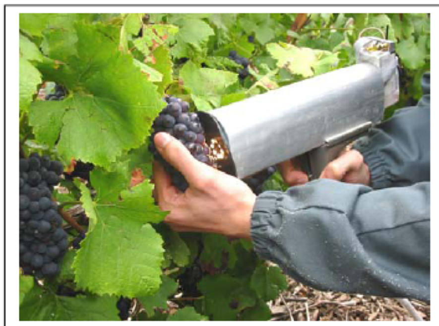
Figure 3.3: Example of an NIR 'gun' under development for the analysis of within-field grape quality pre-harvest (Courtesy of Michel Crochon, CEMAGREF, France)
