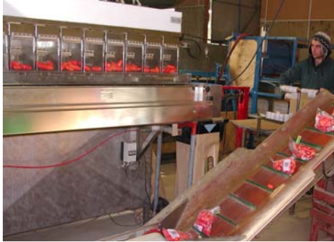
Left: The Halford's new machine which can do 500 g yam prepacks. Right: 9 kg bulk yams.
