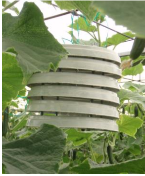
Figure 9 Modified Stevenson screen housing Tinytag Plus 2 data logger in cucumber crop on Northern Adelaide plains
