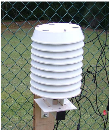
Fig. 5.4.1 Stevenson screen containing temperature and relative humidity sensors
