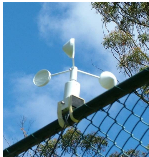
Fig. 5.4.2 Wind speed anemometer
