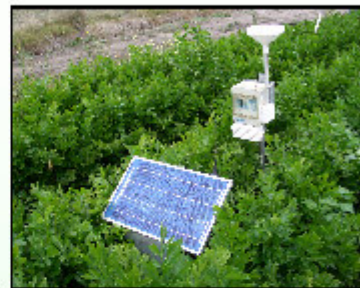
Figure 2. A weather station used in this project. In the foreground is the solar panel unit which also contains the modem and transmitter for sending telemetry via the mobile phone network.
