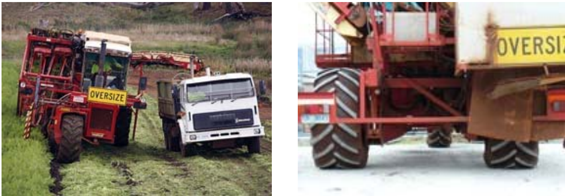
Fig 2. Front and rear views of tri-cycle carrot harvester showing wheel arrangements that are incompatible with CTF.
