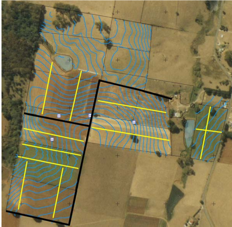
Fig 10. Suggested layout within the constraints of existing infrastructure showing access roads (black) and direction of operations (yellow).
