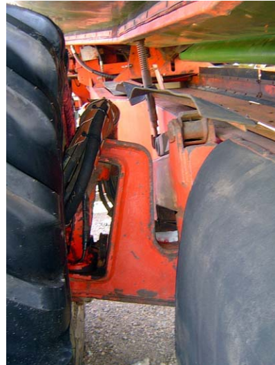
Fig 3. Pea harvester (above) and view showing tyre clearance and construction of axles (right) that limits options for modification for CTF
