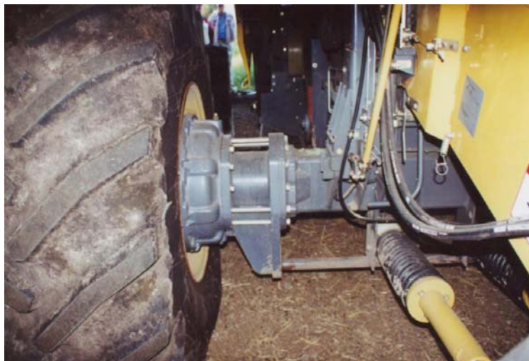
Fig 4. Grain harvester axle extension (3.2 m - 4 m) to allow straddle of 2 m raised beds
