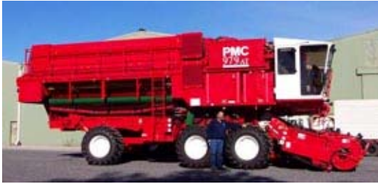
Fig 3. Pea harvester (above) and view showing tyre clearance and construction of axles (right) that limits options for modification for CTF
