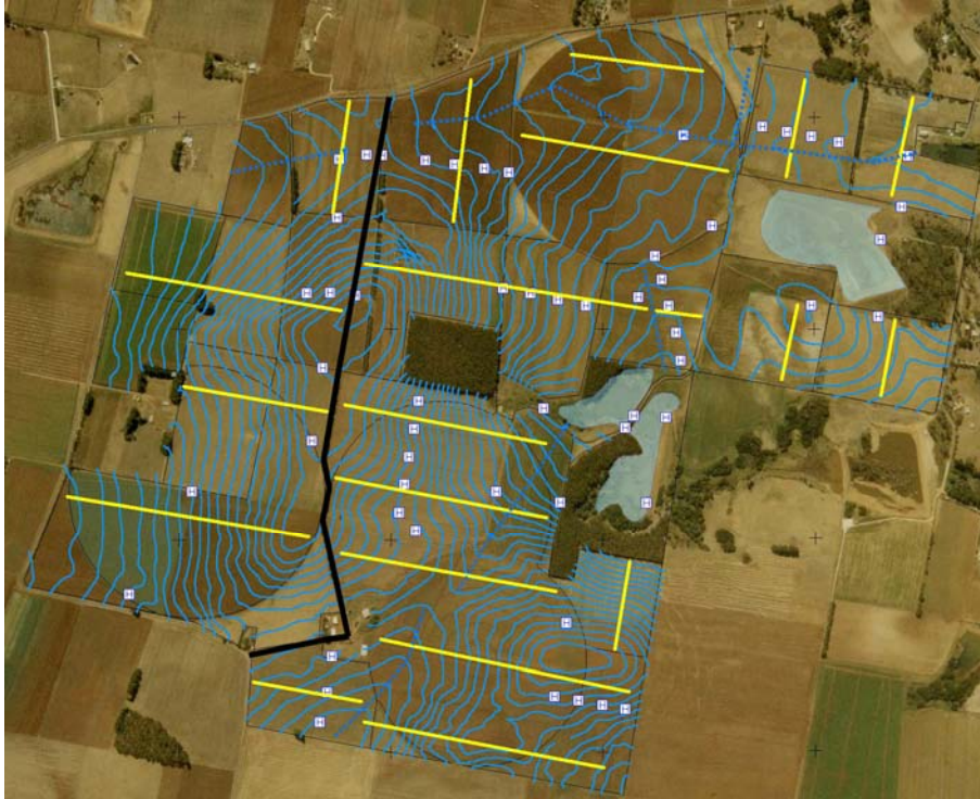
Fig 7. Suggested layout within the constraints of existing infrastructure showing access roads (black), direction of operations (yellow) and drains (blue).
