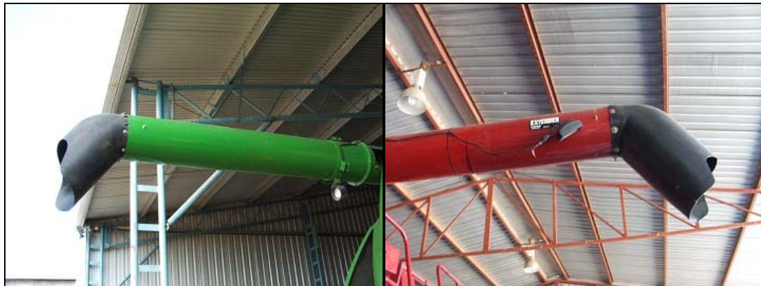
Fig 5. Grain harvester auger extension to allow adequate reach to the chaser bin when on 3 m CTF tracks
