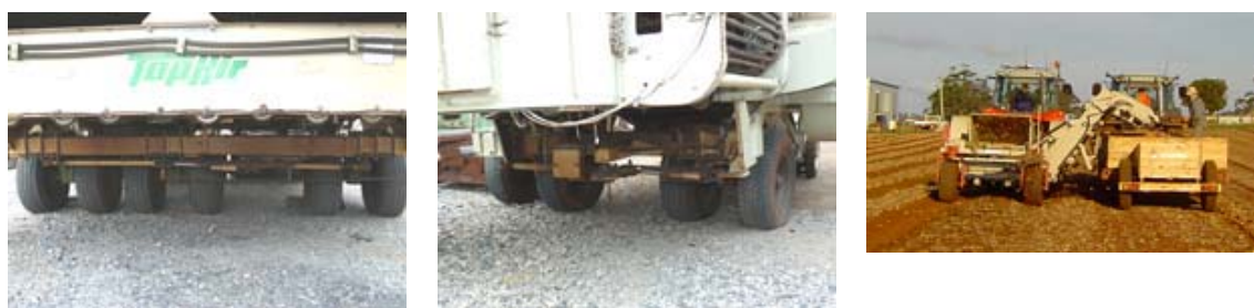
Fig 1. Different tyre configurations for current Top Air twin bed (left), single bed (centre) and alternative style single bed (right) onion harvesters
