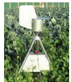
Figure 10. Spore trap for use with the in-field test kit.
