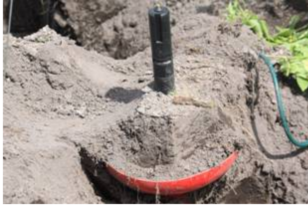
Figure 3-8 Shallow (15 cm) FullStop® showing lettuce root growth in and around the unit and water sampling tube on the right.
