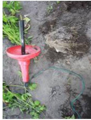
Figure 3-8 Unit removed after crop harvest. Note roots had grown into the buried unit.
