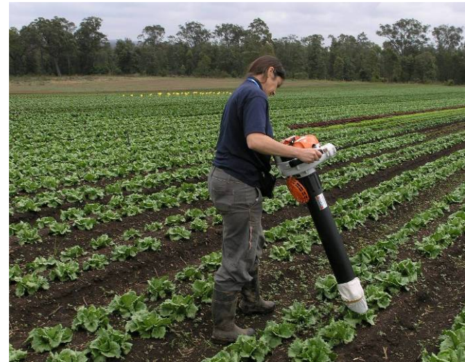
Sandra McDougall demonstrating the bug-vac or vacuum sampler.
