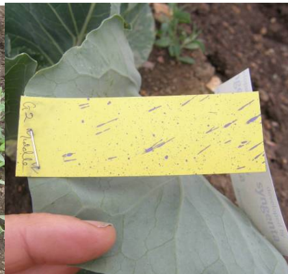
Under lower leaf- poor coverage
