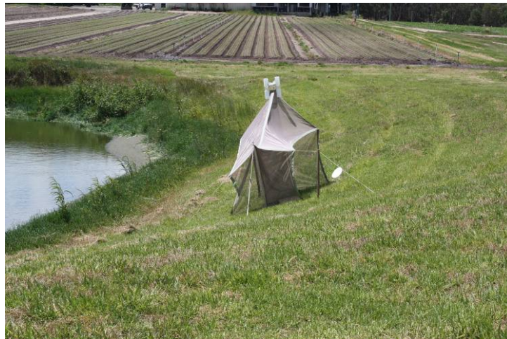
Malaise trap placed in the crop area to sample passing insect flights. Insects caught separately on either side of the trap.
