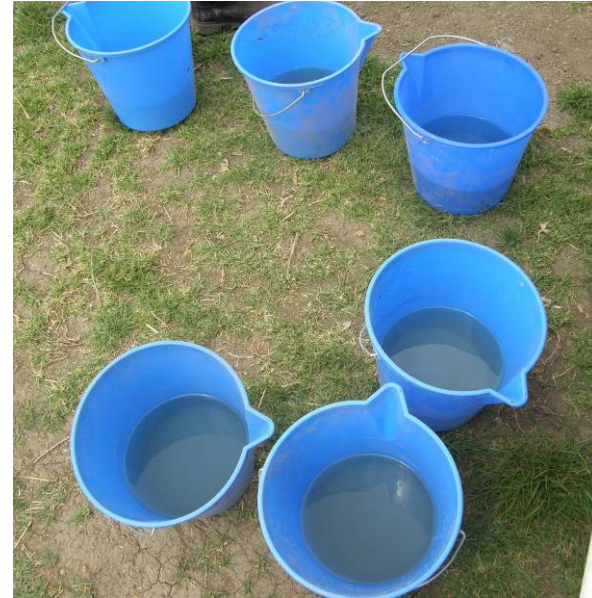
Bucket collection from boom calibration
