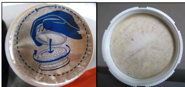
Authentic Original - A pattern of wax dots can be seen both on the seal and inside the cap, due to the Induction Heat Sealing process used at Manufacturing Plant.
