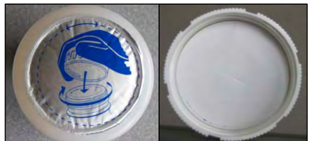
Counterfeit - No pattern of wax dots can be seen - These containers were not sealed by induction.
