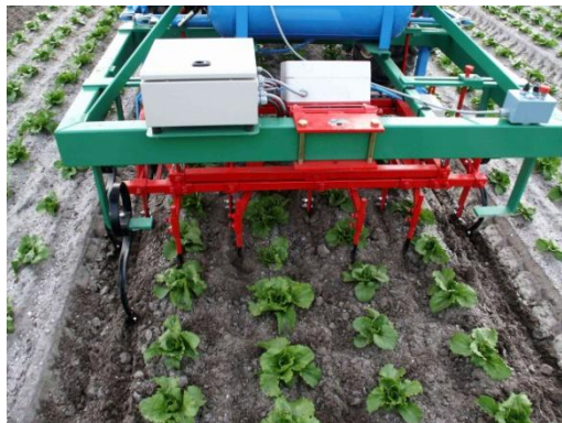
Fig 5.2 Sarl Radis camera guided intra-row weeder.
