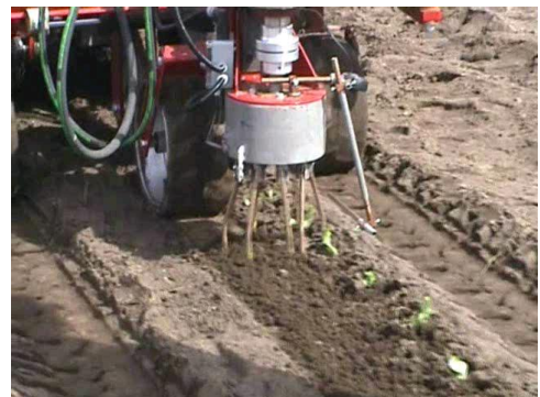
Fig 5.2 Sarl Radis camera guided intra-row weeder.
