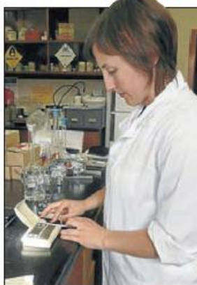
Visiting the Gosford Primary Industries Institute from France, student, Marine Sanoulier, uses test strips with a reflectometer to measure nitrate from leafy vegetables in solution.
