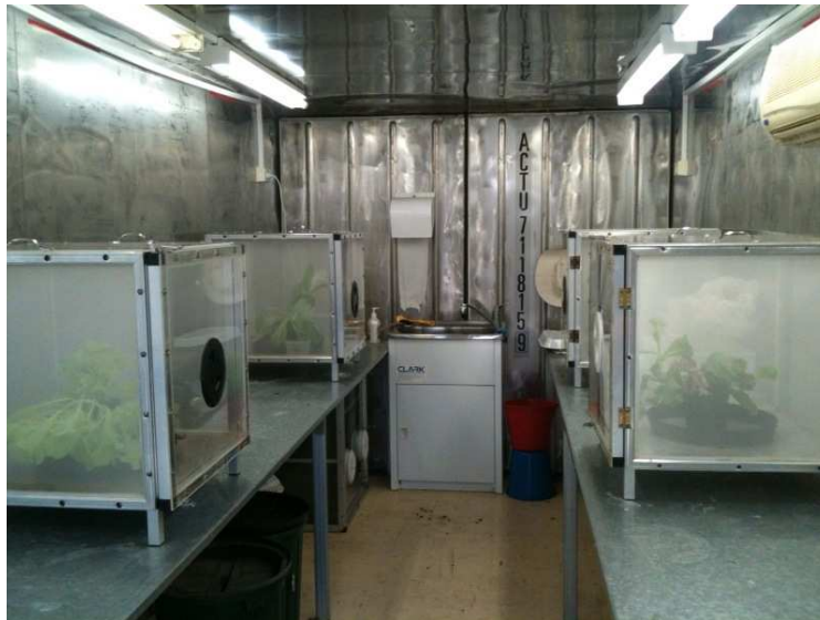
Figure 6. CLA infested plants maintained in insect proof cages at 21°C under fluorescent light
