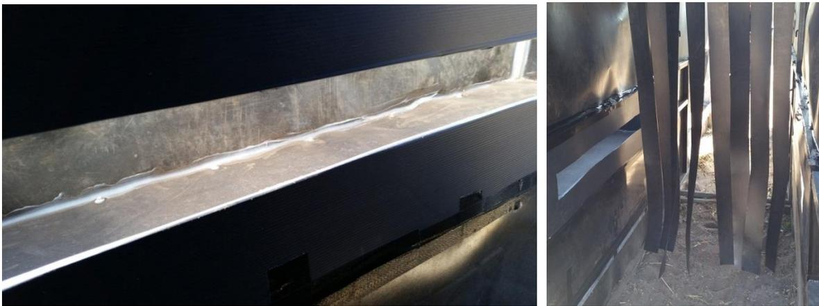
**Figure 19. The third cattle walk-through fly trap design with more concentrated (narrow) light entrance into the side window for capture (L) and the rubber strips on the inside of the cattle trap to help physically remove stableflies from the animals (R).**
