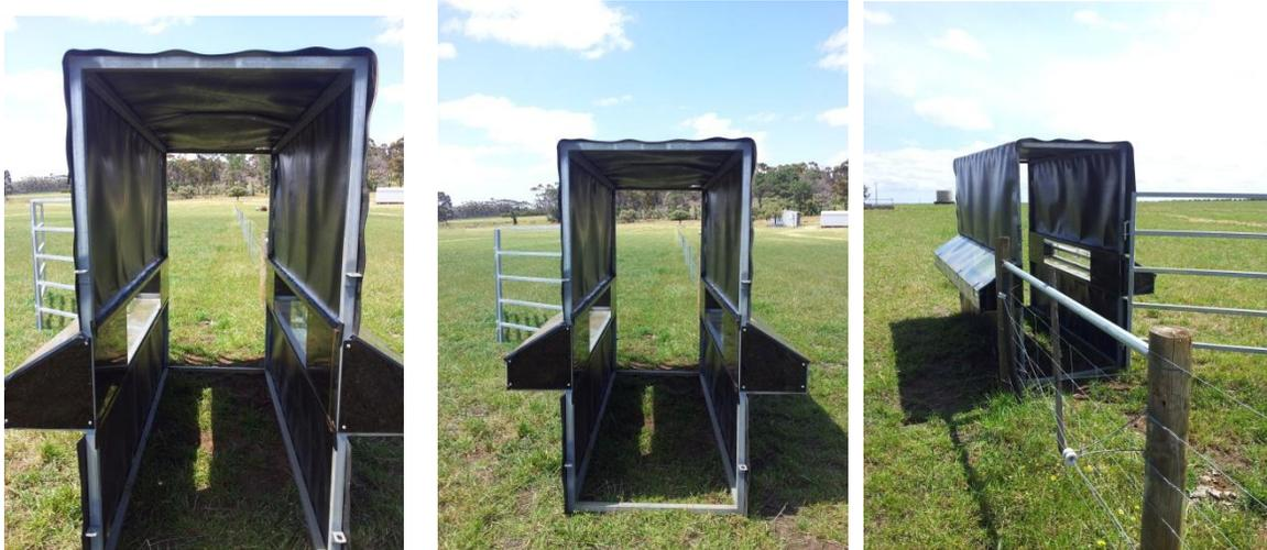
**Figure 16. The first cattle walk-through fly trap design made by DSY Engineering (Muchae, WA) for catching stablefly off cattle placed in the field (Gingin).**
