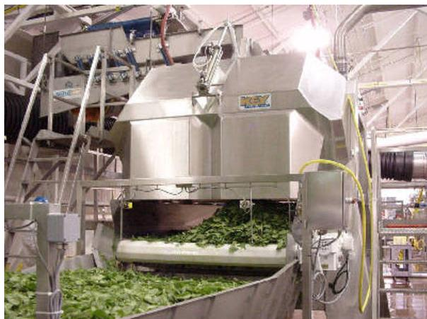
Figure 62 Drum processor
