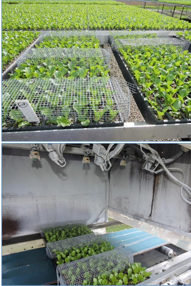
Figure 1 Trial setup showing trays and cages to contain the moths and the spray application setup
