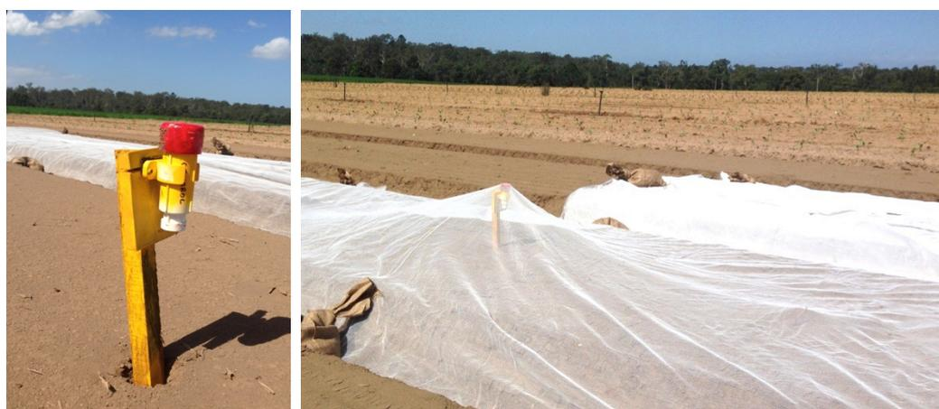
Figure 31 Hobo data logger installed in the open, uncovered area of the bed and under a floating row cover
